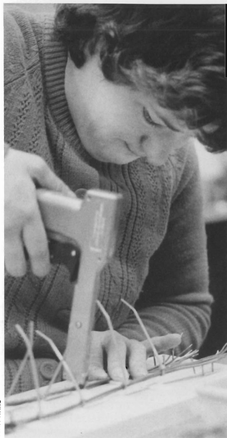
Using a cable gun, Olympus' Shelley Williams tightens cable assemblies that will be used in Lake Stevens products.
